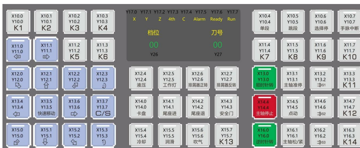
Fig. 3-2 Addresses of Independent-Key Machine Tool Panel (15-inch)
